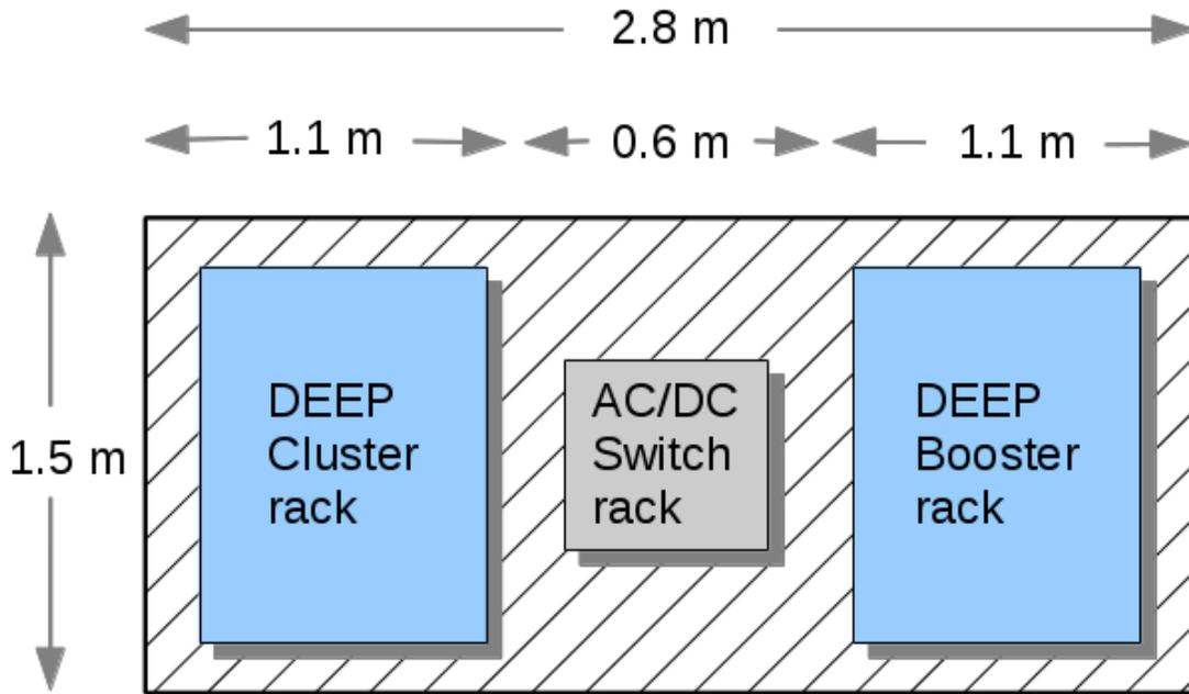
**Figure 2: Floor Space Requirements for the DEEP System**
