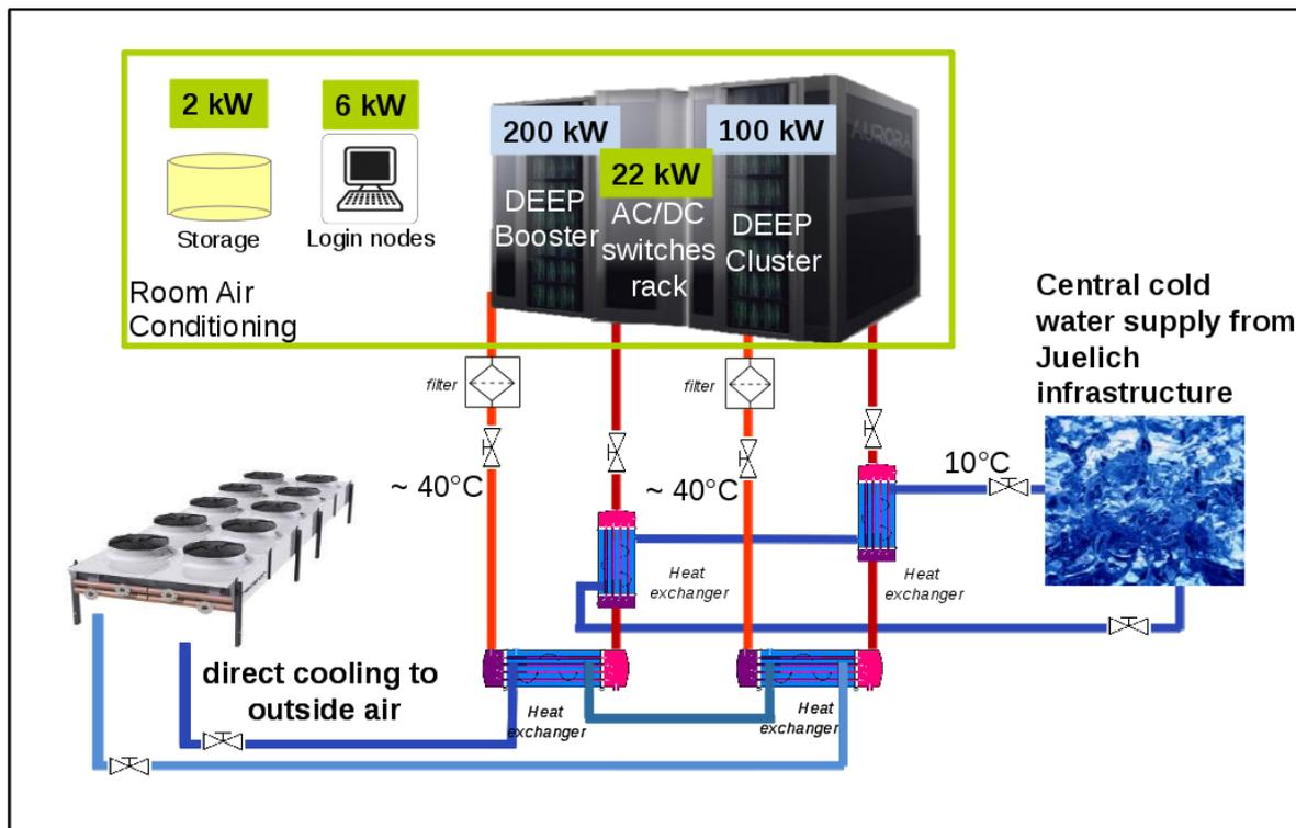
**Figure 1: Cooling Concept for the DEEP System**
