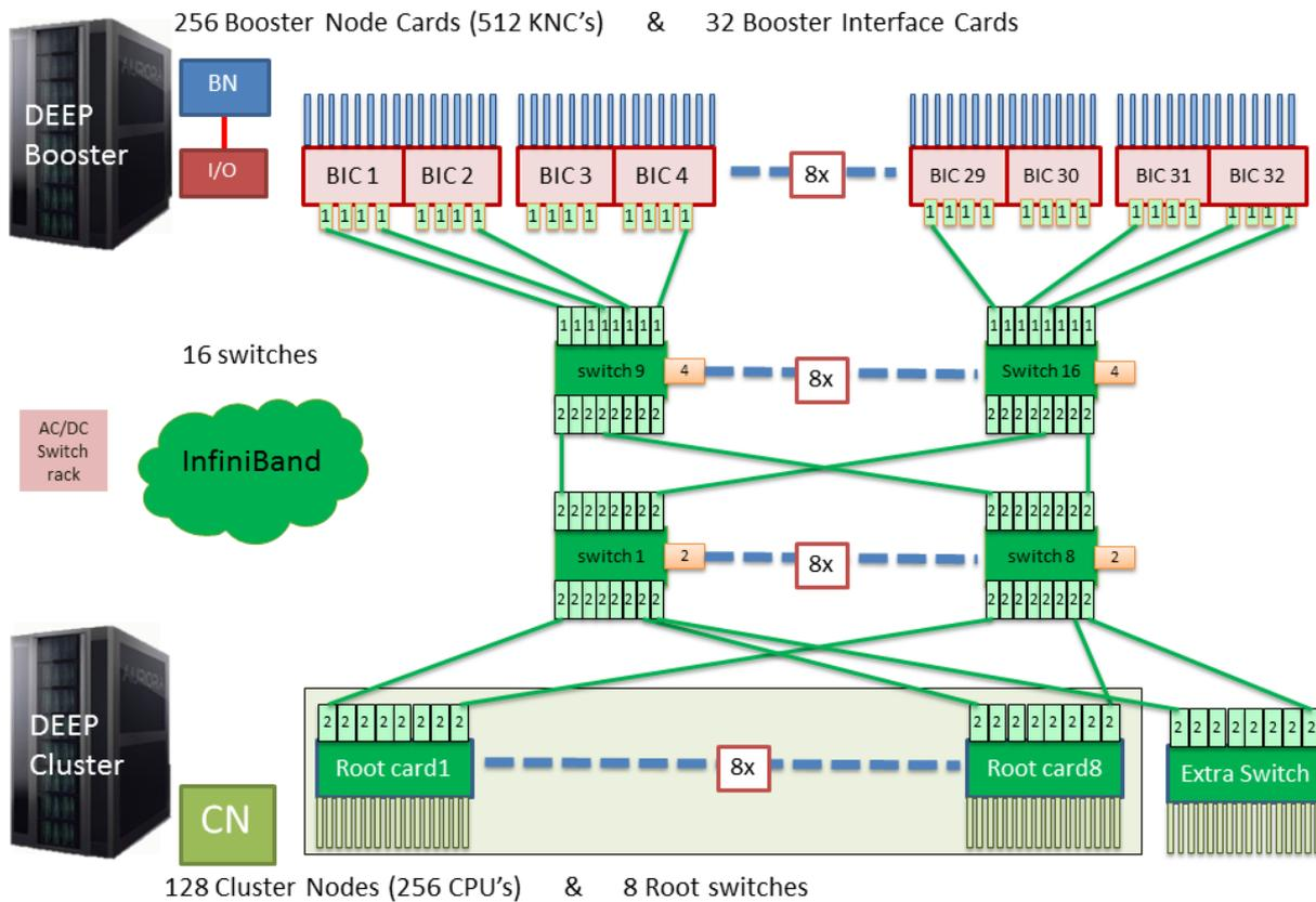
**Figure 5: DEEP InfiniBand Network**
