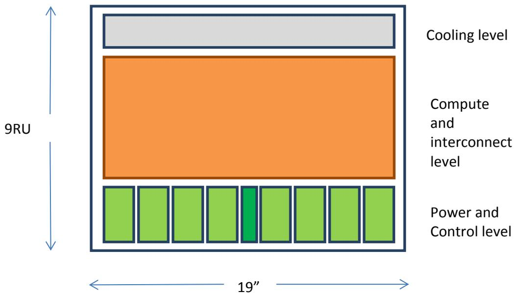
**Figure 4: Levels of the GreenICE chassis.**
