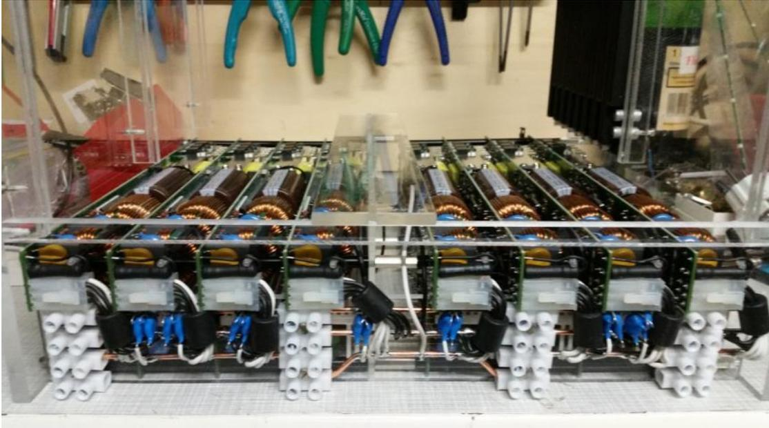
Figure 5: Power supply level showing 8 PSUs
