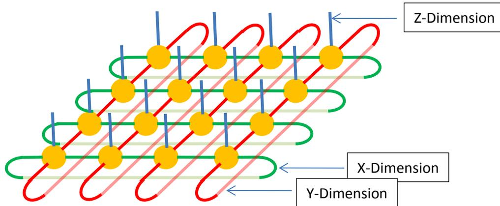
**Figure 3: Lower layer of 3D Torus.**
