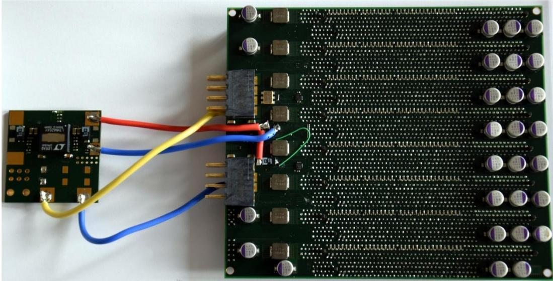
Figure 10: DBP and 12V to 3.3V DC/DC converter on additional board
