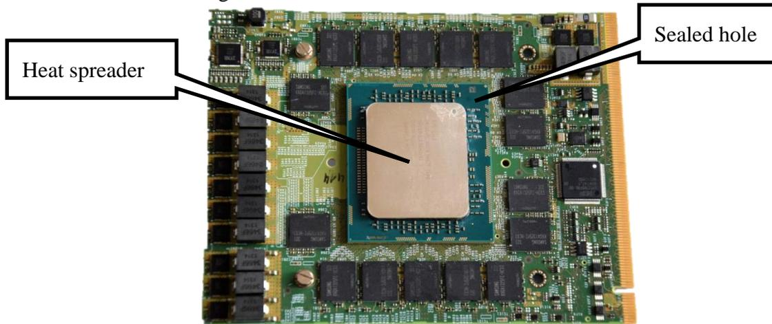
Figure 9: Dense form factor KNC with sealed hole.
