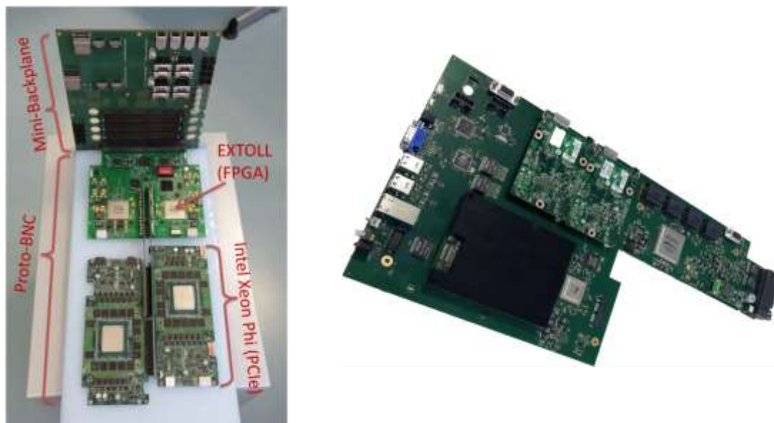
Figure 4: Left: Photo of a BNC Evaluator Board (bottom) connected to a mini-backplane. Right: BIC prototype board, built for the Proto-Booster.
